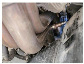
(Note that you are aiming to approximate the OEM distance from the head flange to the o2 sensor. A talented welder can do this on the truck through the wheel well if needed, otherwise the headers must be removed to make the modification.)
