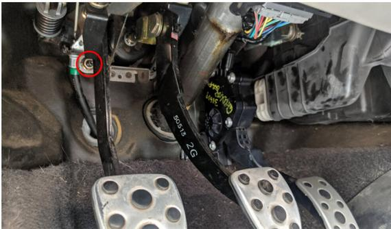
14. Using the supplied 3M tape and zip ties, secure the control box and all wiring out of the way of the shifter and all pedals.
