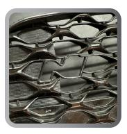
5. Secure the logo to the grill by placing some hot glue or caulk on the backside of the grill to prevent the logo from falling forward out of the grill.
