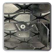
4. Using a dremel, clear out the indented space that the OEM badge was sitting in. Do not remove the raised edge around the outside.
