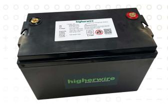
Designed to be discharged to 100% of the rated capacity, this battery is maintenance-free for life. It is a quarter the weight of lead-acid, lasts more than twice as long, and has a flat voltage curve. For maximum cycle life, we recommend keeping charge and discharge below 25 amps, setting charge to 28.0 volts with no equalization, discharging to 24.0 volts and operating above freezing temperatures.
