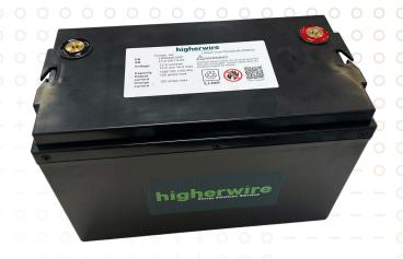
Designed to be discharged to 100% of the rated capacity, this battery is maintenance-free for life. It is a quarter the weight of lead-acid, lasts more than twice as long, and has a flat voltage curve. For maximum cycle life, we recommend keeping charge and discharge below 50 amps, charging to 13.6 volts, discharging to 12.0 volts and operating above freezing temperatures.
