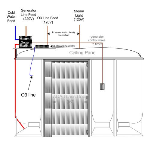
The POWERZONE SHOULD ONLY BE ACTIVATED WHEN THE STEAM/SAUNA ROOM IS UNOCCUPIED. Activate the POWERZONE <u>ONLY</u> during a time when the STEAM/SAUNA room is closed to customers. At least 30 minutes should laps before bathers return to the Steam/Sauna room.
