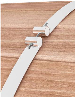
At this point, the metal strap should be wrapping the whole sauna. Place the bolt in the hole located at the tip of the metal strap. Place the washer and the nut on the bolt and fasten them. Make sure you don't over-tighten the bolt. Tap the Staves with a rubber mallet until the sauna forms a well-shaped circle. Adjust the metal strap using locking pliers and an adjustable wrench. Repeat this process with the second metal strap.
