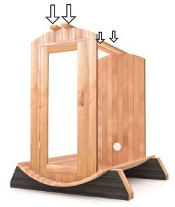
Place the Back Right Panel on the right side of the Central Back Panel. Slowly and carefully, lean the panel (diagonally) and insert it starting from the bottom. Work your way up the groove until both sides are connected. Make sure the bench brackets are facing the inside of the sauna.
