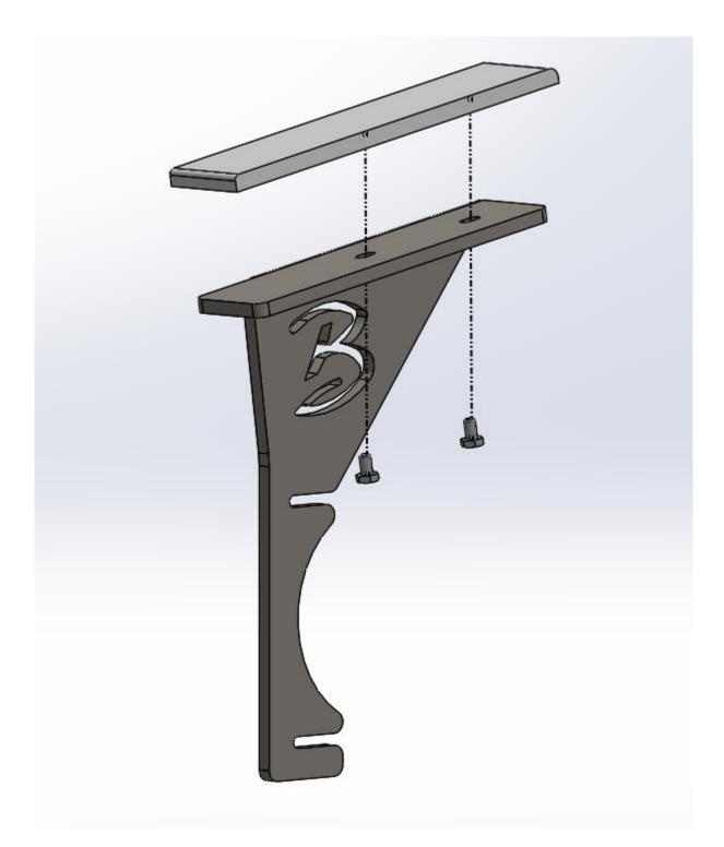
Install the Wear Plate onto the Base using the  $1/4-20 \times 1/2$ " Hex Bolts. The wear plate can me rotated 180 Degrees to use the radius on the opposite end. The wear plate comes from our factory with a 1/8" and a 1/4" radius (one on each end).
