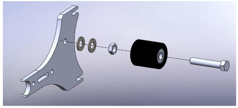
Install the Rubber Wheel (item 2) into the Small Wheel Base (Item 6) using ½" X 2-3/4" Hex Bolt(item 3), Nylock Nuts (item 4) and SAE Flat washers(item 9).
