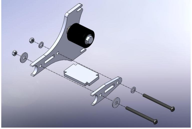
Install the brace (item 1) and side plate (item 5) using the long 5/16" screws (item 7), washers (item 10 & 11), and nuts (item 8). Be sure to install the fender washers (item 11) on the front 5/16 bolt to keep wheels from moving side to side. Be sure to snug and not overtighten these bolts. This can potentially cause tracking issues.
