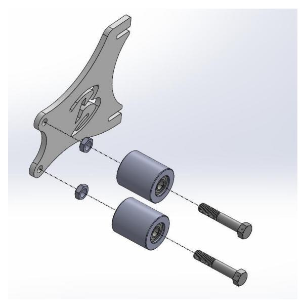
Install the 2" idler wheels into the slack grinding bracket using  $\frac{1}{2}$ -13 x 2-3/4" hex bolt, and nylock nuts.
