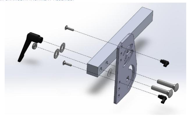
Insert ½-13 x 2.5" Carriage Bolts through the base plate into the arm.
