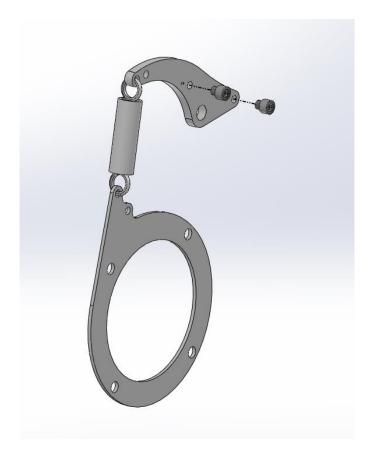
5. Install the  $5/16 \times 1/4$ " Socket Head Screws into the 2 X 72 Coil Spring Tensioner Lever. Connect the spring into the lever and the Coil Tensioner Base as shown.
