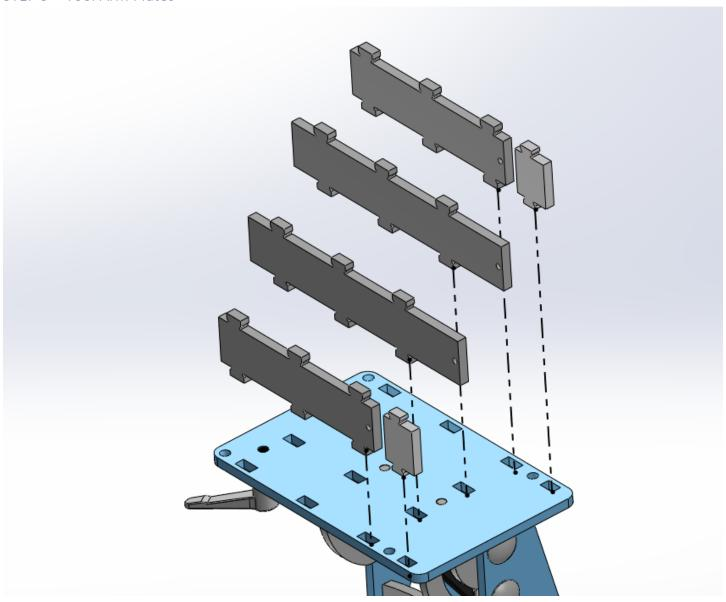
Install the tabs of (in order of front to back) the tool arm top plate, tool arm plates (2), tool arm top plate, and motor side plate stiffener into the slots of the hinge-side side plate.
