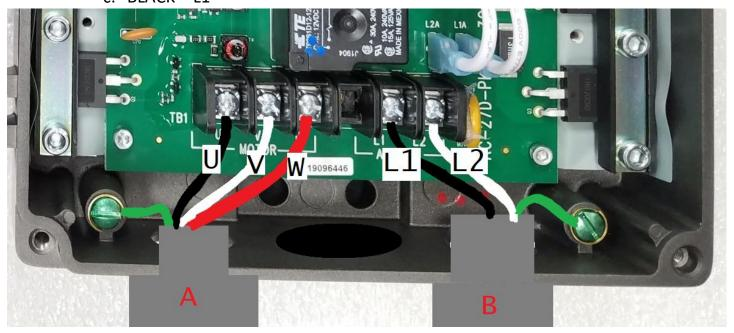
2. Set the input voltage jumper (J1) to the correct supply voltage (230V shown in photo). Standard Household voltage is 115
