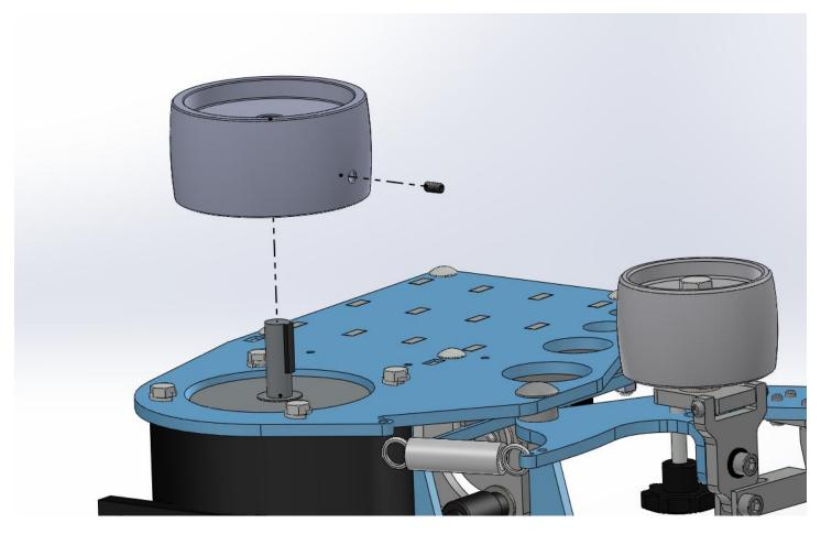
Align with other wheels to ensure proper tracking. The drive wheel should be 7/16" off of the side plate.
