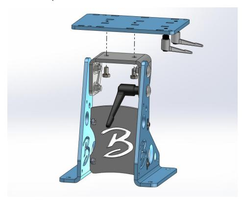
Lower the hinge-side side plate onto the hinges. Use two  $3/8-16 \times 5/8$ " Long hex head bolts.
