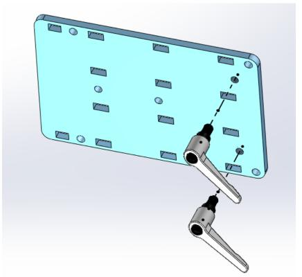
Install the 3/8-16 Threaded Handles into the Hinge-Side Side Plate. Do not tighten down all the way. Only tighten until the tip of the threads meet the inside face.
