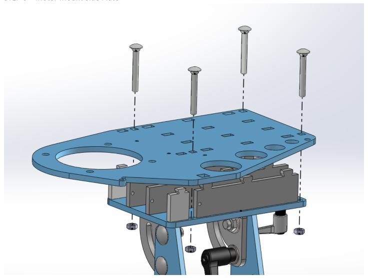
Place the motor mount side plate onto the tool arm and tool arm top plates.
