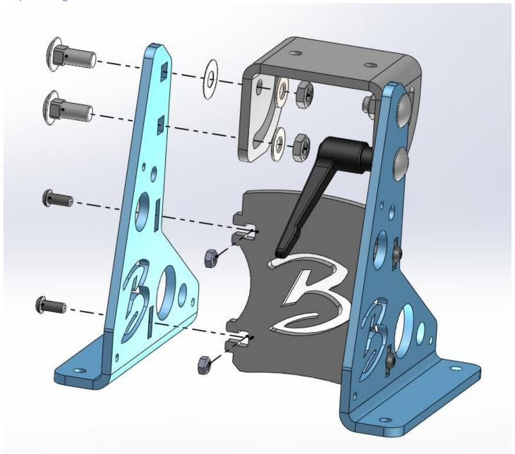
Insert a 1/2" x 1-1/4" long carriage bolt into the top and bottom hole of the Hinge Base. Then add a 1/2" teflon washer (.020" thick) to the top bolt. Install the Hing Base onto the X-Brace and Hinge. Then add a 1/2" metal flat washer and a 1/2" thin nylock nut. Tighten until you can barely rotate the hinge.
