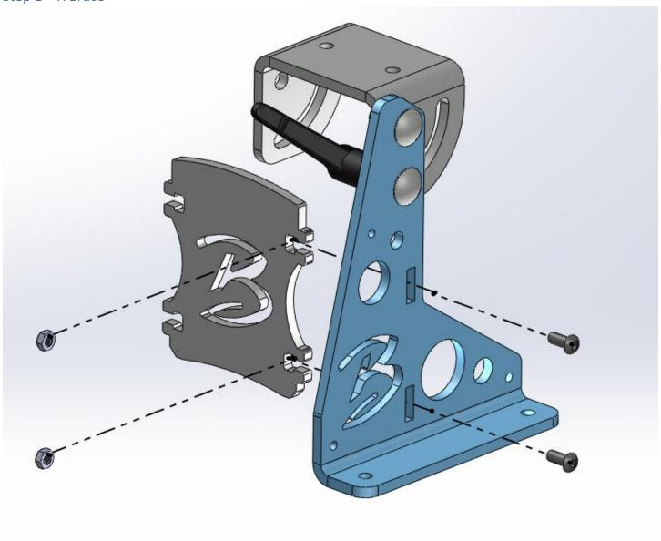
Insert X-Brace into the Hinge Base. Slide 5/16-18 nylock nuts into the X-Brace. Secure with  $5/16-18 \times 3/4$ " long Button Head Screw by inserting it through the Hinge Base into the nylock nut.
