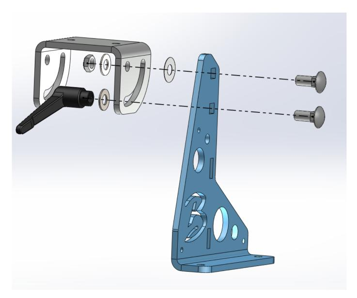
Insert a 1/2" x 1-1/4" long carriage bolt into the top hole of the Hinge Base. Then add a 1/2" teflon washer (.020" thick) to the bolt. Add the hinge on top of the carriage bolt. Then, add a 1/2" metal flat washer and a 1/2" nut. Tighten until you can barely rotate the hinge.
