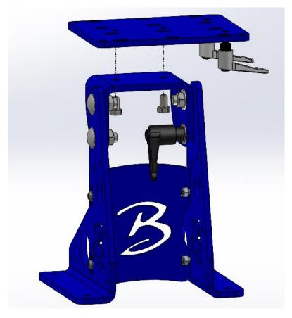
Lower the hinge-side side plate onto the hinges. Use two 3/8-16 x 5/8" Long hex head bolts.
