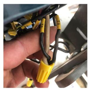
5. Connect T2 and T8 to the 4 conductor cable red wire.
