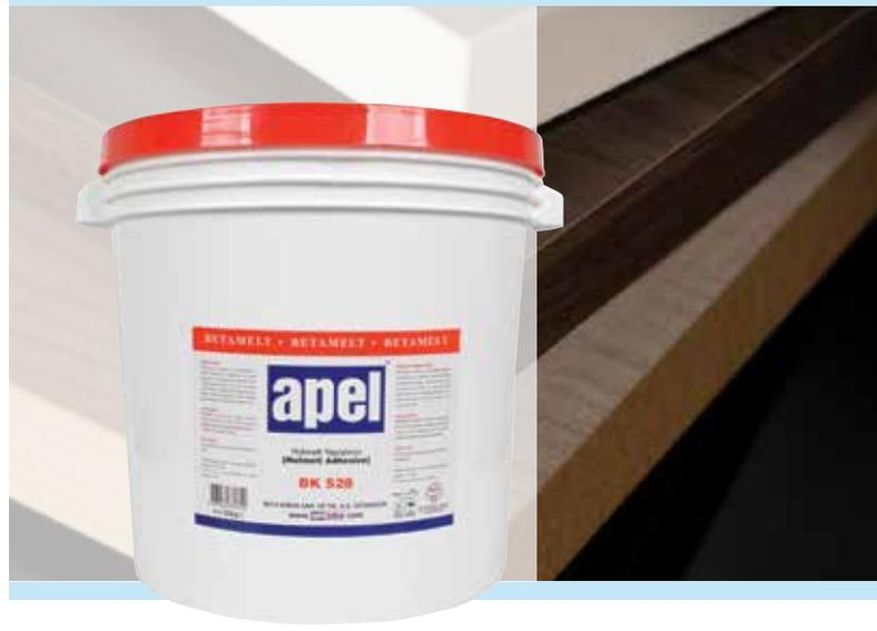
Apel BK 528 is a natural colored edge-banding glue with medium open time and excellent final bonding. It is specially formulated for medium speed (12 - 18 m/min ), roller-press, automatic straight edge-banding machines. It can be used to bond wood, PVC, melamine, ABS edge-bands to MDF, chipboard or solid wood boards. Not suitable for acrylic edge-bands.
