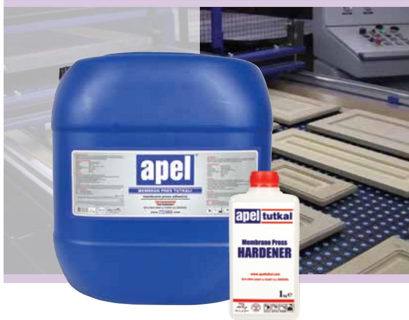
Apel Membrane Press Glue is water based dispersion adhesive that is used in automatic vacuum membrane press machines for bonding PVC membrane foils to MDF. There are two types of this glue as a single component and two component choices. The two component glue is used with a hardener with a specific proportion (%5) to receive a higher temperature resistant after cured.
