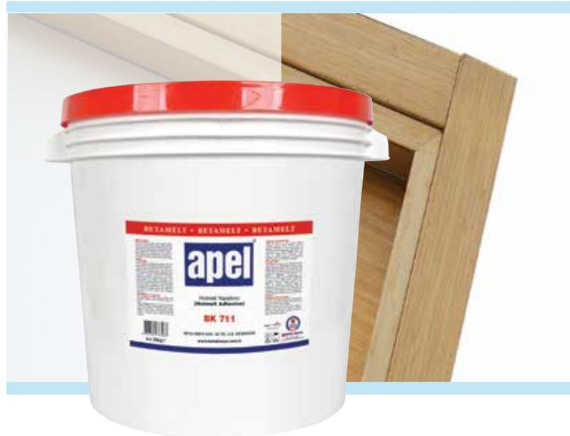
Apel BK 711 is an EVA based granule hotmelt glue, produced of high quality synthetic resins which is used for bonding solid MDF materials in door frame production industry. The glue has a low/mid viscosity values, good surface wetting ability and high thermal resistance. It is mostly used for bonding MDF pieces in automatic door jamb bonding machines in high temperatures. For an optimum bonding quality, the machine speed is suggested to be 15 m/min.
