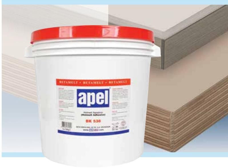
Apel BK 538 is a semi-natural colored edge-banding glue with long open time and excellent final bonding. It is specially formulated for low and medium speed (8 - 12 m/min) automatic edge-banding machines. It can be used to bond wood, PVC, melamine, ABS edge-bands to MDF, chipboard or solid wood boards. Not suitable for acrylic edge-bands. Good price/performance ratio.
