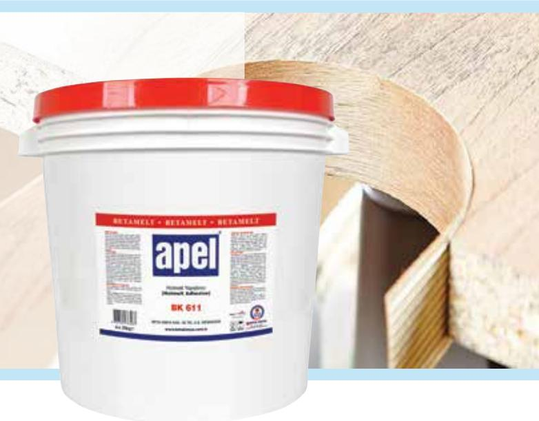
Apel BK 611 is an EVA based, low viscosity, granule hotmelt adhesive which is specially formulated for low speed (8 - 12 m/min) and/or low temperature linear and nonlinear edgebanding applications. It is produced of high quality synthetic resins and best used for to bond PVC, melamine, ABS, polyester, laminate edgebands to surfaces like MDF, chipboard and solid wood materials.
