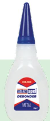
Mitreapel Debonder is used to uncure and dissolve cured instant adhesives and glues and remove the undesired residue of these chemicals. Debonder must be directly applied on the surface of the residue and let it set for 1-2 minutes, then must be cleaned with a fiber cloth or paper towel.
