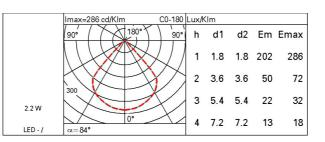
ballast Vin=100-240V ac - Light Blade optic (Up) + Wide Flood optic (Down)
