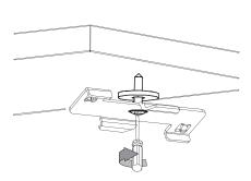
**Step 3**Attach surface mount bracket to ceiling using screw and washer provided.
