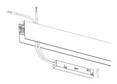
**Step 1**Snap Live end connector into track light and thread through rear of the track.
