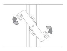
**Step 5**Rotate surface mount bracket to align with snap track, should click when properly fastened
