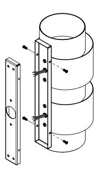
Attach the wall plate to the wall using 4 x screws suitable for the surface you are mounting to (not supplied), ensuring that the electric cable is centred with the hole in the middle of the wall plate.
