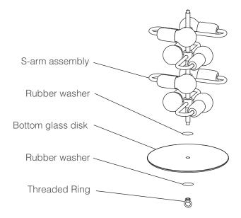
Using the below diagram and the labeled glass, hang the vertical glass disks on to the cross-member's arms.
