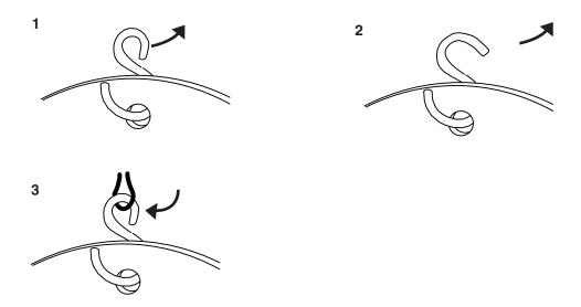
Using a pair of pliers, carefully open the glass mounting hooks ( $\mathbf{1}$ ) wide enough to fit the pin, attached on the frame ( $\mathbf{2}$ ). Fit the hooks to the pin and carefully close the hooks with the pliers ( $\mathbf{3}$ ) taking care not to damage the glass or the fitting.
