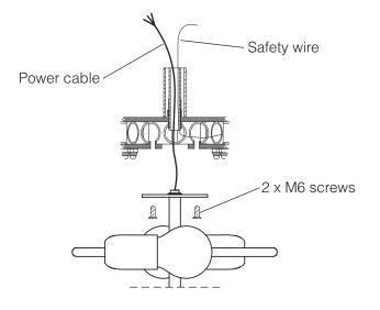
Screw the ceiling back plate to the ceiling. Ensure that suitable screws are being used for the surface you are mounting to.
