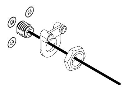
**6.** With the base securely fixed to the bottom of the stem, remove and replace the screws and clamp on the cable clamp.
