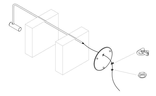
**5.** With the base positioned on the end of the stem in the correct orientation, move the cable clamp into place and secure with the hex nut.
