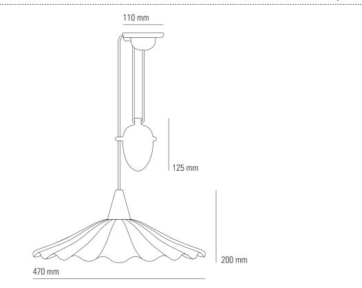
Cable length may be shortened upon installation. This will reduce both maximum & minimum drop and reduce the range of movement.
