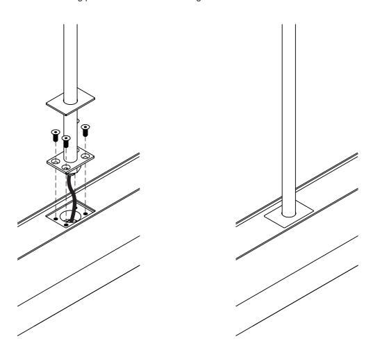
2. Securely fix the mounting plate to the ceiling in the correct position using fixings suitable for the surface you are mounting to (not supplied).
