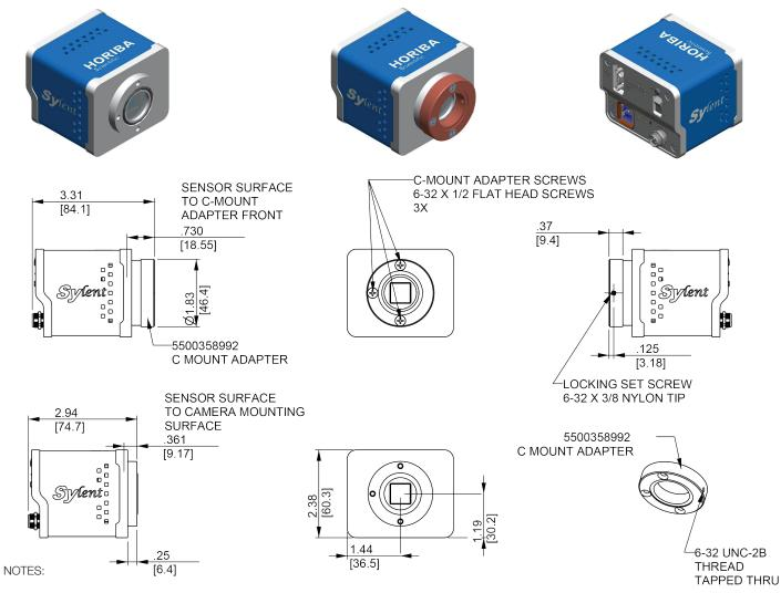
1. UNITS ARE IN INCHES [MILLIMETERS] UNLESS OTHERWISE NOTED. 2. AVAILABLE ADAPTERS: C-MOUNT, F-MOUNT AND CUSTOMIZABLE
