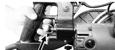
Pull release pin to rotate handle.
