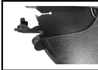
Figures 9a and b. Dust cover removal after releasing magnet on dust cover.
