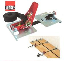
No. SVH-400 157" Flooring Strap Clamp w/Spacer (13' 1") No. SVH-760 300" Flooring Strap Clamp w/Spacer (25') Used for installing parquet, plank hardwood, laminate and other tongue and groove flooring. The ratchet action of the clamp pulls boards together and keeps them tight, providing up to 220 lbs. of clamping pressure. Each Clamp has 15/16" wide high strength polyester strap, spacer and galvanized or painted parts to resist rust. Clamp plate is 43/4" wide x 31/2" deep.
