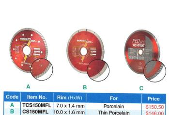
10.0 x 2.4 mm Thick Porcelain, Granite The No. TCS150MFL Blade (f A) is supplied with the No. MOTO-300-FL Flash Line System. All three blades have a 6" diameter, are the Montolit Red Line 'Professional' Series with arbor sizes of 1/6" and 11/6", and are suitable for dry use. The Nos. TCS150MFL (f A) and TBH150 (f C) Blades are a Turbo Rim type. The No. CS150MFL (B) Blade is a Continuous Rim type.
