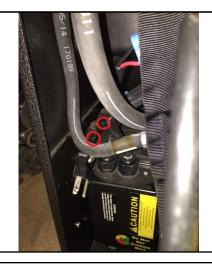
To remove the mounting screws: (1) Remove the front screw first; allow the charger to pivot down. (2) Ensure fingers are not under the charger, then remove the back
