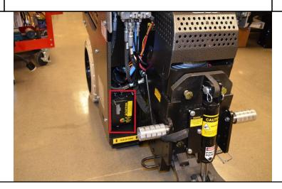
Unplug the black connector with the orange and yellow wires from the black connector with the black and white wires.
