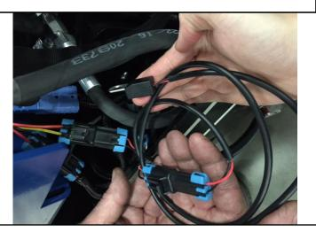
Run the thermal probe behind the hoses and harness, under the metal bar and wires, then over the second bar 38 and up to the negative battery terminal with the black boot and zip ties
