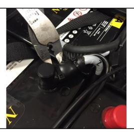
Unscrew bolt and place thermal probe.
