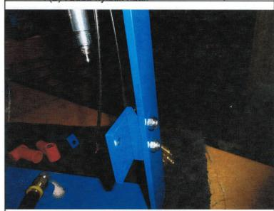
Get regulated elbow from Propane Kit. Loosen locknut. Tighten needle valve until lightly seated. Loosen needle valve 5 full turns. Tighten locknut
