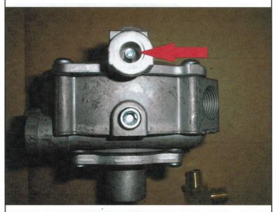
Assemble bushing and regulated elbow from Propane Kit to OUTLET of propane regulator. Use teflon tape to seal parts.
