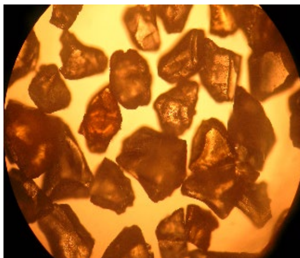
Figure 1. Appearance of EXFO-AMBER (X 10) observed through an optical microscope (Unilux-12, Kyowa)
