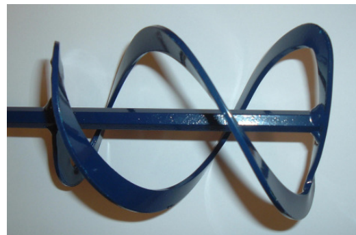
Figure 3: Mixing equipment (cement mixer, l = 14 cm) to homogenize TEGOSOFT® LSE 65 K soft (mainly before analytical tests)
