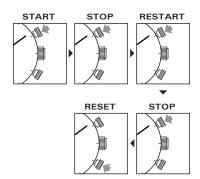
Restart and stop of the stopwatch can be repeated by pressing the button **A**.
