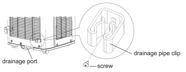
2. Remove the rubber plug at drainage port.
