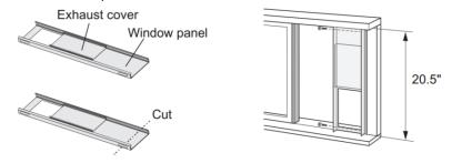
Inner height of the window:20.5" (520mm)- 38.5" (980mm) Use the window panel and the adjustment panel.
