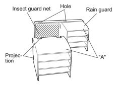
2. Attach the guard combined above to the window panel. Push the insect guard net firmly to ensure that its four projections fit into the holes in the window panel. Side "A" will now be at the top, as indicated in the diagram.
