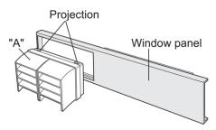
3. Cut the sponge A (adhesive type) to the proper length and attach it to the window stool and to the bottom of sash.
