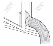
4. Slide and open the exhaust cover on the window panel and attach the window adapter.
