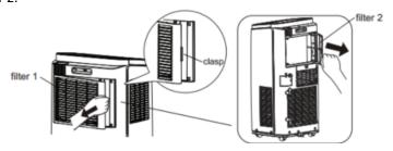
2. Clean filter: use cleaner or water to clean the filter. If the filter is very dirty, use warm water melted with neutral abluent to clean it and then put in a shady place to dry.
