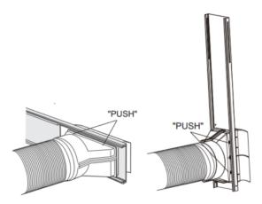
2. Remove Joint: Press the clasp and lift Joint upwards to remove it.
