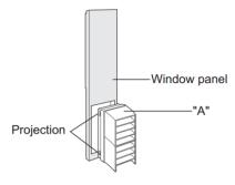
3. Cut the sponge A (adhesive type) to the proper length and attach it to the window frame and to the side of sash.
