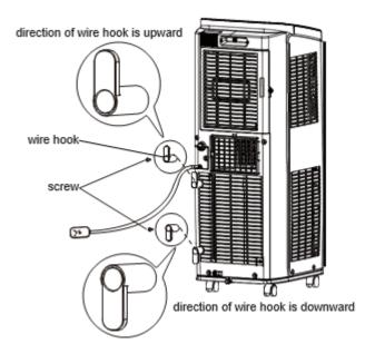
2. Wind the power cord around the wire hook.
