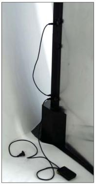
**STEP 7**Connect the fan unit by the cord and attach the foot pedal
