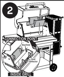
Install heat deflectors on both sides of the manifold.
