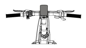
**Step 5.** Release the clamp under the handlebar, pull the handlebar up or push it down to adjust height to your desired, then close the clamp to secure handlebar in place.
