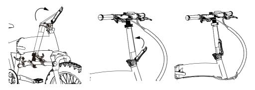
**Step 3.** Stand in front of the bike and clamp front wheel between both legs, verify the handle bars are straight and in line with the front wheel. Make sure the pinch bolts are tight and your cannot turn the stem freely from the front wheel. Sit on the saddle, adjust the handlebar to comfortable angle, and close the handlebar
