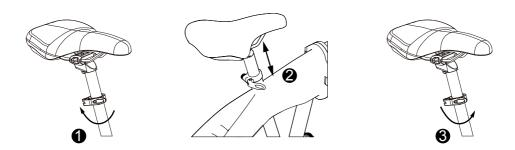
**Note:** Position the seat at the right height is key for better pedaling, safety and overall comfort. The rider's leg length is used to determine the seat's position. When pedaling, your hips should remain level and your legs should not over-extend. To determine the right seat height, sit on the eBike with pedal at its lowest point and place the ball of your foot on the pedal. If your knee is bent slightly at this position (about 60 degrees), the seat is at the right height.
