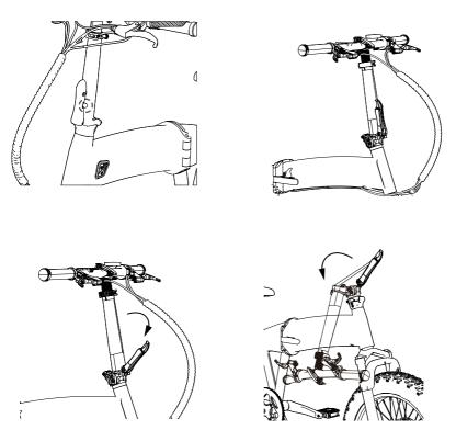
4.To fold the frame, pull the metal safety lock towards to front of the bike. While pulling the safety lock, pull the Latch outwards. When the latch has been released, fold the bike.
