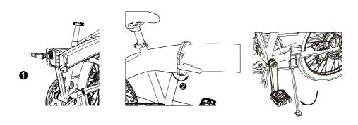
Step 2. -Pull the stem upright and fold the latch up to close it.
