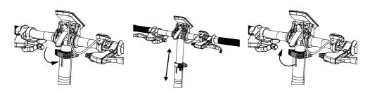
**Step 6.** Open the clamp under the seat post,set it to a height which fits the rider then close the clamp to secure the seat in place.
