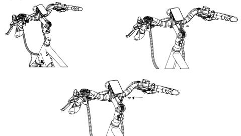
C. Center the handlebar and screw in the four stem faceplate bolts evenly, however do not tighten all the way down for further adjustment.
