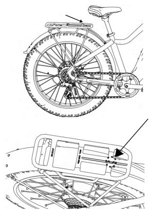
E. Check the bottom screws and make sure they are fixed.
