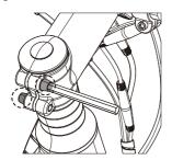
D. Adjust display to the desired position, tighten the screws with 2mm hex key.
