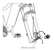
D. Use 15mm open wrench to tighten front axle nut, recommended torque value at 25-30Nm.
