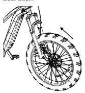
B. Remove fork protective cover and take out plastic insert from front wheel brake caliper.
