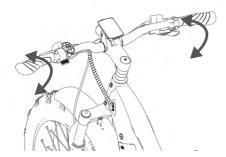
B. Stand in front of the bike and clamp front wheel between both legs, verify the handle bars are straight and in line with the front wheel. Make sure the pinch bolts are tight and you can not turn the stem freely from the front wheel.
