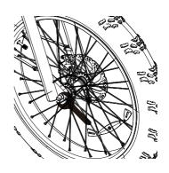
**Caution:** Never touch the brake rotor, especially when the wheel and/or bike is in motion, or serious injury could occur. Hand oils can cause squeaking and decrease brake performance
