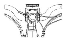
E. Adjust the head light to desired position, tighten the screw with a 4mm hex key. Loosen the circled screw if you want to adjust the display's angle.
