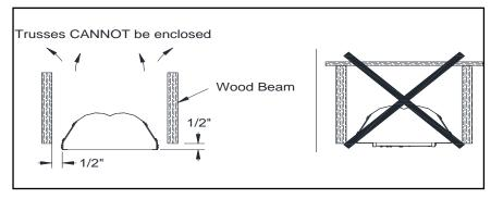
The heater can be mounted in a variety of ways, using a combination of chains and mounting bracket. It is critical that the heater is prevented from swaying and putting stress on the gas connection. Also, be sure to check local codes for seismic bracing requirements for outdoor heating equipment.
