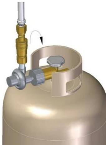
Figure 11: Secure Gas Regulator to Propane Cylinder
