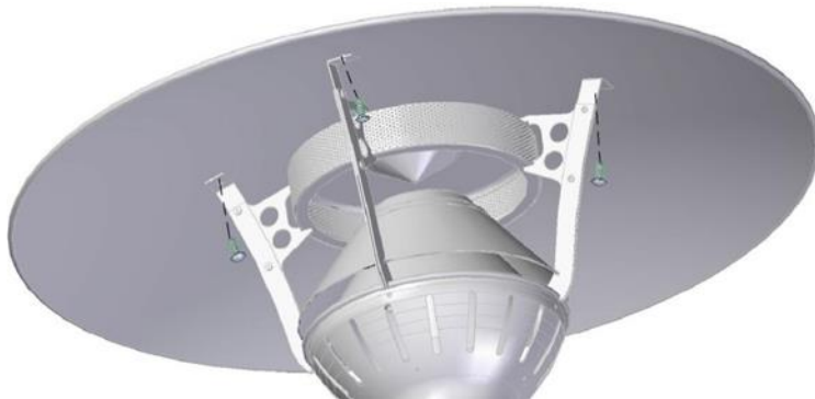
Figure 7: Attach Top Reflector to Shield Support Arms
