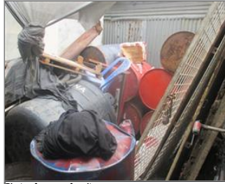
Photo of non-conformity Wastage without segregation.JPG
