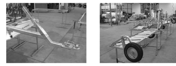
Fit the drawbar. Fit and plumb tank if required. Adjust the suspension, outer wheels and drawbar to suit the operation.
