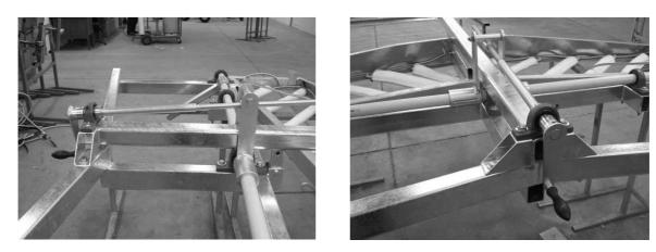
Bolt the pillow block bearing to the frame and bolt the "T" piece to the quadrants.
