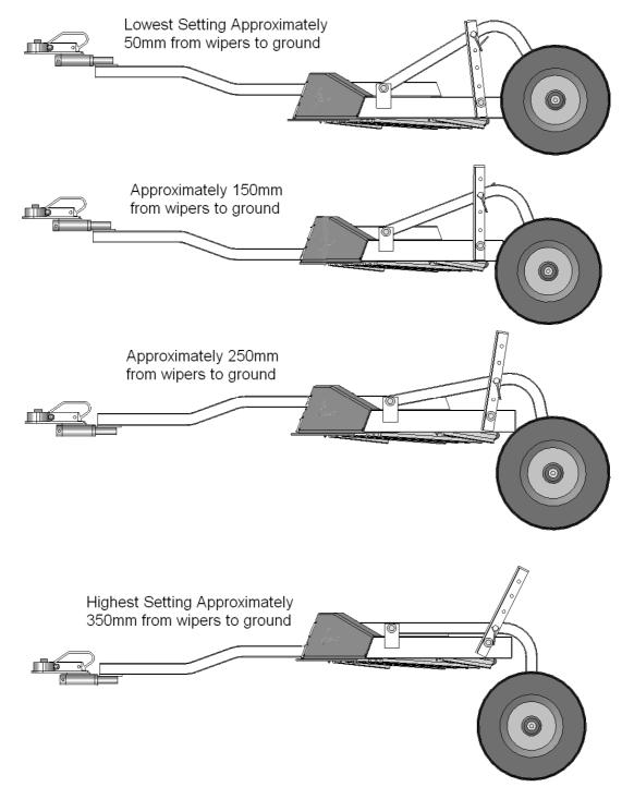
On the Winged Eliminator unit the wings are self angling and as such the unit can only be set approximately level when the height adjusters are on the second hole from the top.
