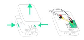
Open Enegic Monitor by pressing both sides together and pulling up the lid.
