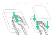
Anchor the cables with the included cable ties and guide them out the cable grooves.
