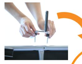
Order of insertion screws (a), flat washers (b), brake (c), plastic washers (d), trailer structure (e), antivibration washer (f) and plastic-wing nut (g)
