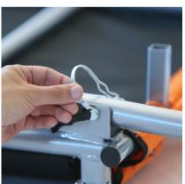
Insert the metal pin in the correct orifice and clip it to secure the towing arm in place.
