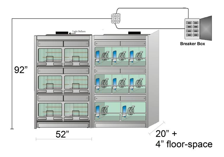
Each 2 unit set-up requires one electrical quad-box outlet centered between the units. The middle of the quad-box outlet needs to be 92" off of the floor. Each unit uses 2 amps of energy. The quad-box outlet needs to run of one 20 amp breaker.
