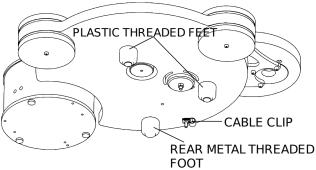
Set the plinth height by rotating the 3 adjustable feet. It helps to lift the deck slightly for access to each foot in turn
