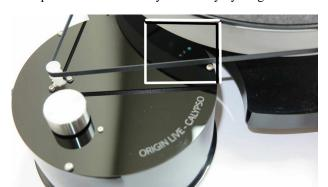
reading the speed of the platter. You will notice 3 closely spaced holes near the edge of the motor pod. These holes house the light emitters and sensors that read platter speed and must be positioned under the rim of the platter as shown in photo below.
