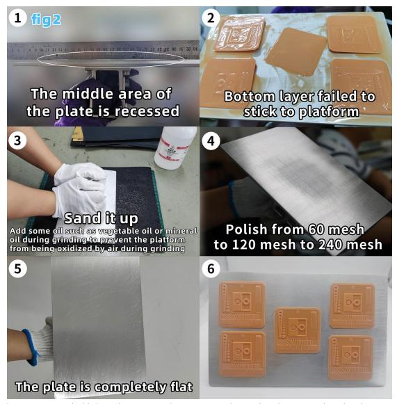
b.Use a magnetic build plate. The magnetic plate is too smooth to stick to the prints and needs to be removed or use 800 grit sandpaper to roughen the magnetic platform before use
