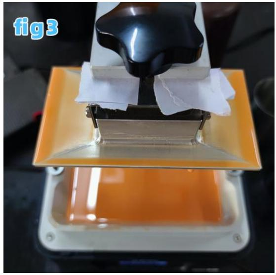
After eliminating the above problems, you can start setting parameters and slicing. We recommend using the "Rest time after bottom retract" Setting, set 8–10S. It is more conducive to the bottom layer sticking to the build platform.
