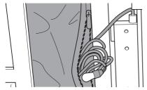
The power cable can be placed in the pocket beside the door for storage.
