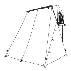
The awning is attached to the poles of the roof tent with clips. After the awning has been fastened and aligned, it is secured to the ground with pegs.
