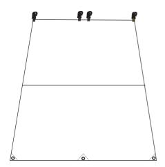
The awning is attached to the poles of the roof tent with loops. After the awning has been fastened and aligned, it is secured to the ground with pegs.
