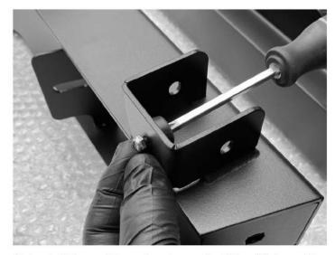
6. Install the rubber stop to each of the (4) legs. Use (1) 6-32 x 3/4" machine screw and (1) 6-32 nylon lock nut for each stop.
