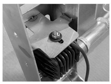
9. install (4) 2" LED lights into legs as shown using 8mm x 25mm hex bolt, flat washer and lock washer.
