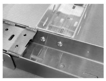
5. Connect second side of both of the lateral cross bars to the transverse cross bar as shown. Use (2) 3/8"x1" button head bolts and flange lock nuts. Torque to 30 ft/lb.
