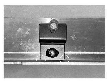
11. Install the assembled rack to the vehicle. Do not install the clamps until after the rack is on the vehicle. Center the rack in the bed, using the (6) rail brackets clamp the bed rails to the vehicle. NOTE the chamfered corners of the bracket install to the rail first, then fasten the clamp bolt to secure the rail to the vehicle.
