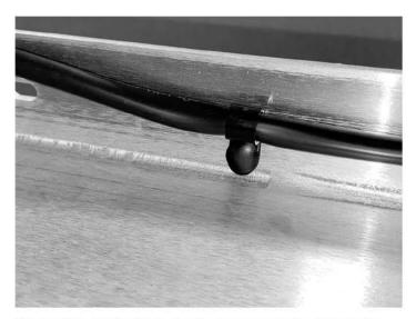
10. Route LED wires and harness on the right side of the vehicle using supplied wire clamp and push rivits as shown on the inside of the bed rails and cross bar assembly. Each leg and transverse cross bar has (9) holes, Each base rail has (7) holes.
