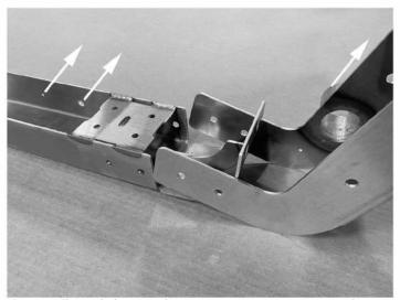
1. Install each leg to the transverse cross member. Use (6) 3/8"x1" button head bolts and flange lock nuts for each corner. Do not tighten securely. Make sure holes on the transverse cross member and gate pivot tube are facing the same direction.
