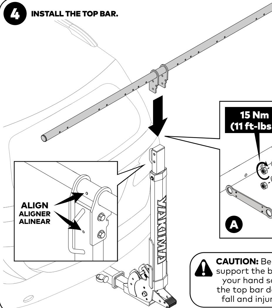
A. Join the top bar to the mast (red dots must be on same side - toward the vehicle). Use the closed wrenches to install the bolts, washers, and hex nuts as shown. Tighten to 15 Nm.
