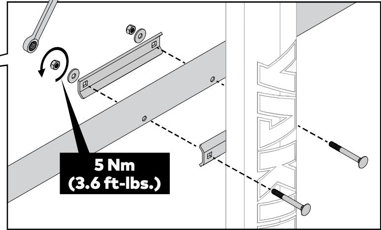
Use the 10 mm wrench to attach the lower bar to the mast with the carriage bolts, plate, washers, and nuts. Make sure that the rivets face outward as shown. Tighten to 5 Nm.
