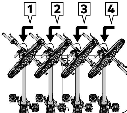
**NOTE:** When carrying 1 or 2 bikes, load them in the positions closest to the mast. Load the bike on the left first.
