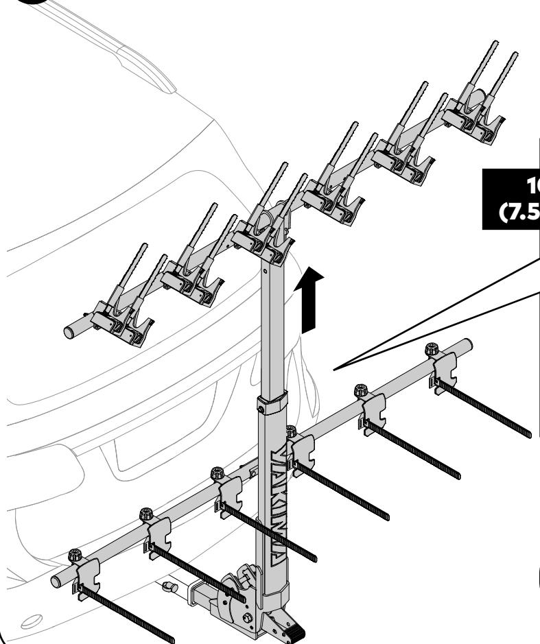
Use the open wrenches to loosen and remove the mast hardware. Raise the mast, align the holes, then reinstall the hardware. Tighten to 10 Nm.
