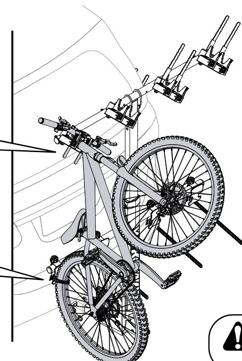
A. Adjust the pads on the strap to cover the handlebar. Route the straps through the buckles and pull down to secure the bike. Make sure the straps are tightened evenly. **NOTE:** Move or remove handlebar or stem mounted accessories if they interfere with the cradle or straps. Avoid securing straps over disc brake lines
