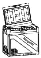
Align the door shaft with the hole on one side and insert it
