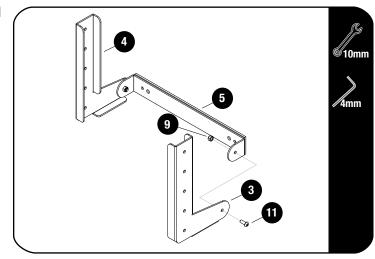
Loosely assemble the LH & RH Side Brackets (Item 3 & 4) to the Swivel Mount Bracket (Item 5) using M6 x 16 Button Head Bolts and M6 Nyloc Nuts (Items 9 & 11) as shown.
