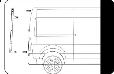
Find suitable rigid mounting points to prevent the door from deforming.
